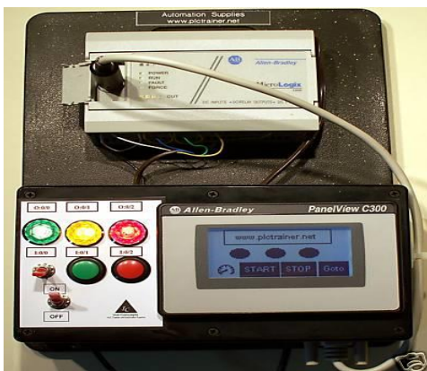
Allen Bradley PLC Micrologix 1000
