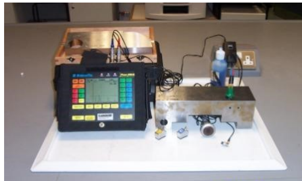
Ultrasonic Testing (UT) Equipment
